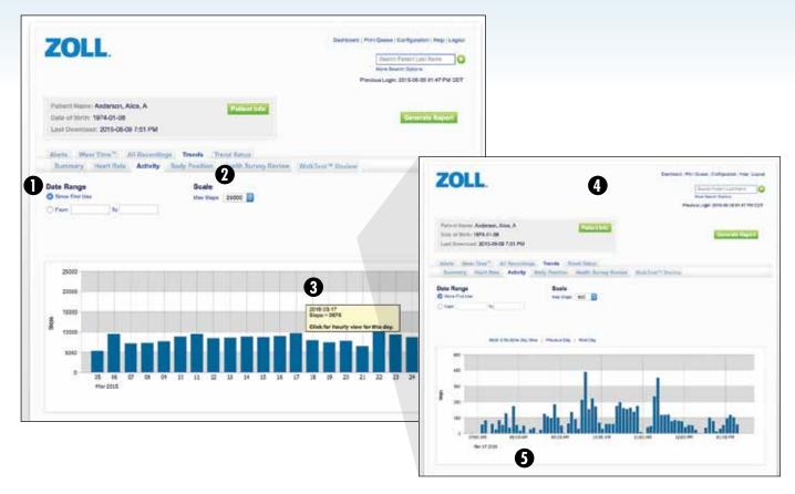
The LifeVest enables you to track trends in patient activity based on patient movement. An accelerometer located in the electrode belt of the LifeVest WCD determines the patient's step count, similar to commercially available pedometers. The data is initially displayed as hours of activity per day. To be counted as an hour of activity, the patient's activity must exceed 120 steps per hour. You can also view the activity by steps.
